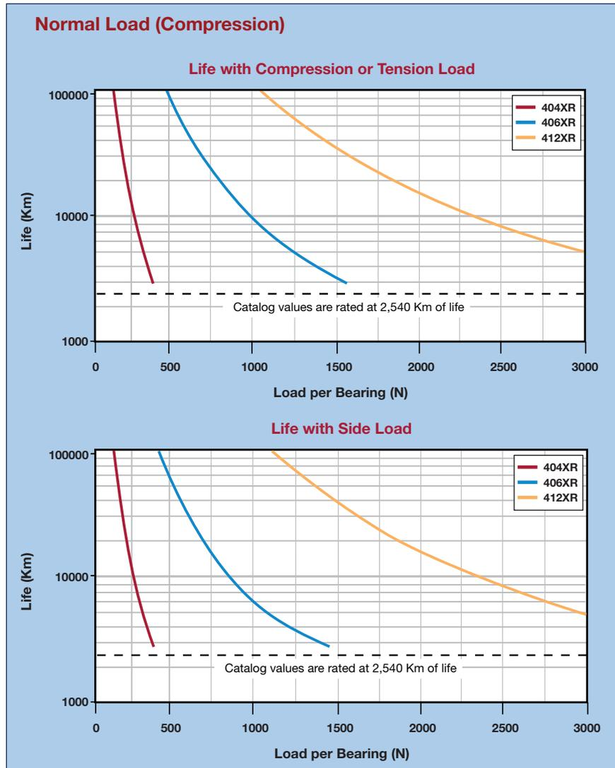
These charts are to be used in conjunction with the corresponding formulas found in the product manuals at [www.parkermotion.com](http://www.parkermotion.com) to establish the life/load for each bearing (4 per table).
