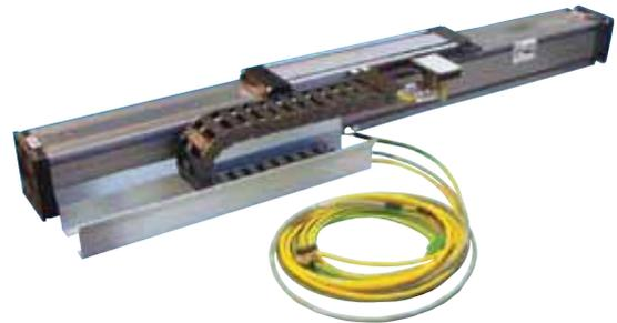
The BLMA is a plug and play linear motor actuator which houses a powerful linear servo motor (386 pounds of peak thrust) in a high strength rigid aluminum body to enable high end performance with highly repeatable positioning over long unsupported spans.
