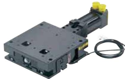
The ZP200 is a unique vertical lift stage providing up to 25 mm lift with no horizontal translation in a small package. The ZP200 uses ballscrew technology and a square rail bearing design.
