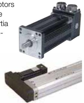
As standard, the motors are offered in an in-line configuration and for space constrained applications, may be mounted in a parallel configuration. The parallel design utilizes a belt and pulley to transfer torque and includes additional pulley support bearings to protect the motor shaft and screw shank from over tension and fatigue failures.
