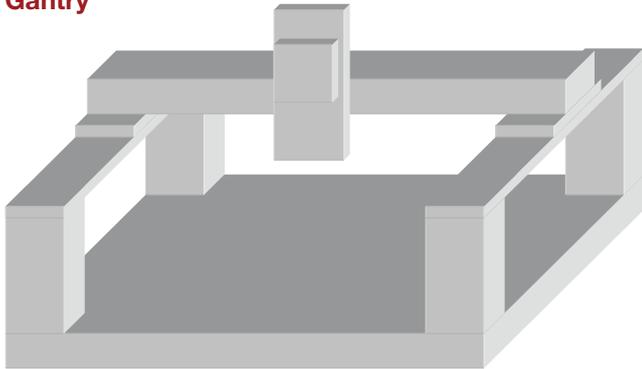
This configuration has the best accessibility to the space around it per footprint of the machine. It is commonly used as single cell or in process application where several machines are operating over a conveyor. Gantry configuration, driven by linear motors and designed for
