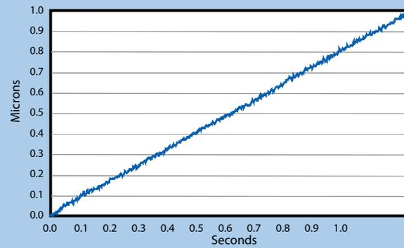
Note: Test were performed using a model MX80LT04D13E8 with a 20 nanometer linear encoder
