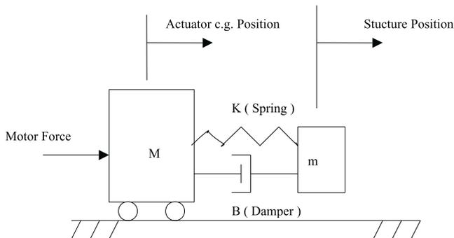
Once the physical model is defined, a schematic diagram shows the main mechanical components, which are included in the theoretical model, and the way they interact. The diagram shows for example a model of a positioning stage with mass M, driven by a motor force and carrying a flexible structure with mass m, stiffness K and Damping B. The schematic diagram is then used for writing the equations of motion of the theoretical model.
