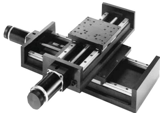
The top and base are constructed of high quality aluminum alloy and are protected with a black anodized surface finish. The top and bottom mounting surfaces are precision ground to assure flatness and all mounting holes are fitted with locking steel threaded inserts to prevent mounting bolts from working loose.
