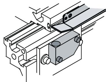
**4-wire NPN switch with mounting hardware**
