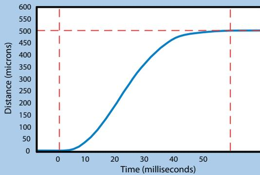
Note: 1 Kg payload, 500 micron move:
