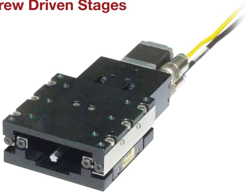
The leadscrew drive employs a PTFE coated leadscrew with a preloaded nut to produce extremely smooth linear translation. A choice of three leads provides improved opportunity for matching desired velocity/resolution requirements.
