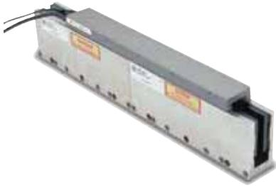
Parker Trilogy's I-Force ironless motors offer high force and rapid accelerations in a compact package. Parker Trilogy's patented I-beam shape, with its overlapping windings, allows for a higher power density in a smaller motor, improved heat removal, and added structural stiffness. A forgiving air gap and no attractive forces allow for easy installation and zero cogging during motion.
