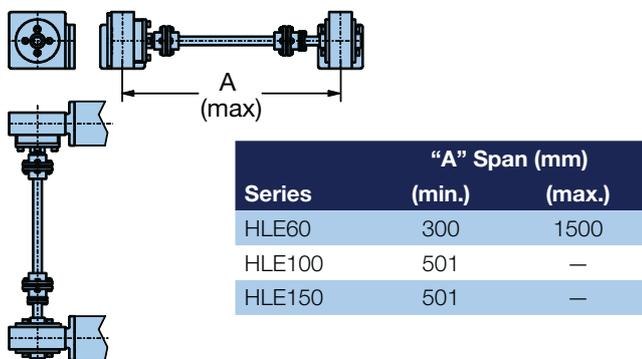
The link shaft bearing is used to support the linking shaft of an HLE dual axis when there is a large center to center distance. This bearing must be used if the critical speed is exceeded with the dual-axis link shaft.
