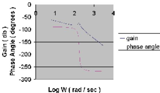
The structure transfer function, has the “stage position” as an input and the actual “structure position” of a point of interest on the structure (e.g. Encoder location) as the output. This is a classical transfer function of a mass, spring, damper system with a positive position excitation of the base.
