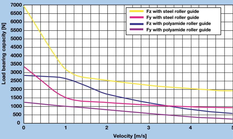
The curves show the maximum load-bearing capacity of a carriage in one direction of force or torque. If several loads are applied in different directions, the values given by the curves must be derated, i.e. the load or speed should be reduced if necessary.
