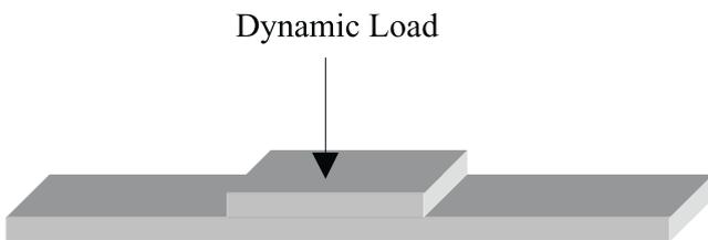
Dynamic loading of a stage is the maximum load that may be applied for a bearing life of 254,000 m (10 Million inches) of travel with no evidence of fatigue appearing in 90% of the bearing. This assumes that the load is constant in magnitude and direction and that all forces are perpendicular to the motion of the stage.
