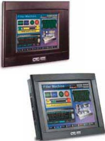
EPX PowerStations provide a bundled Level II hardware and software solution at a price point that is competitive with most Level 1 solutions. EPX PowerStations are available in the following display sizes: 8", 10.4" and 15".
