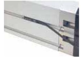
For maximum flexibility, sensors are adjustable over the entire length and magnets are included on both sides of the table so sensors can be attached on either side. The sensors are offered in 4 variants with NPN (sinking) or PNP (sourcing) outputs and in normally open (NO) or normally closed (NC) logic. The sensor cables extend 300 mm and terminate into a M3 connector. If purchased as part of the positioner (LH option) each sensor will include a 5 m extension cable (P/N: 003-2918-01).
