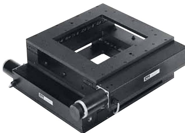
Table elements are constructed of high quality aluminum alloy and are protected with black anodized surface finish. The top and bottom mounting surfaces are precision machined to assure flatness, and fixturing holes are fitted with locking steel threaded inserts. These units are offered in English or metric versions, and in two grades: precision grade and standard grade which permit cost savings to be realized in less demanding applications.
