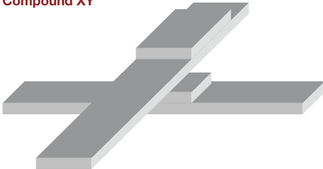
This configuration provides the simplest form of 2 linear degrees of freedom of a positioning system where the base of the top axis is bolted to the slide of the lower axis. For a high-performance positioning application, a “monolithic” design can be used where the base of the top axis and the slide of the bottom axis are rigidly made as a single part. In a compound XY configuration care should be given in consideration to the Abbe Error of the top axis due to cantilever “diving board” effect.
