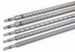
As standard, the HD Series offers 5 mm, 10 mm, and 20 mm lead options with a 40 mm lead available as a special. For most travels, the screws are 15 mm in diameter with the longer 20 mm lead and all 40 mm lead screws increasing to 20 mm in diameter. Like the linear bearings, the screws are self lubricating and will not require re-lubrication for the table's life.
