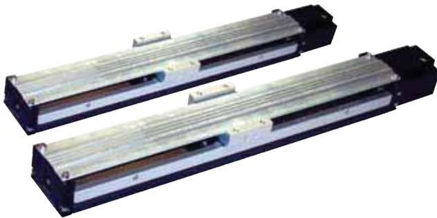
The steel base constructed 402/403XE series offers rigid compact positioning for the cost conscious motion applications. A highly integrated ballscrew, bearing retainer system results in a very low overall height and high payload capacities.
