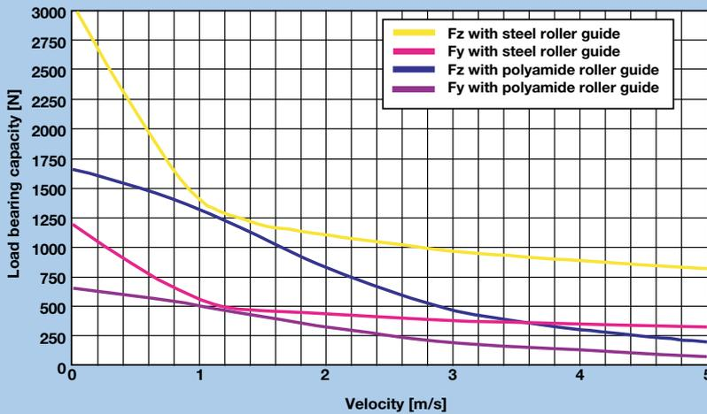
The curves show the maximum load-bearing capacity of a carriage in one direction of force or torque. If several loads are applied in different directions, the values given by the curves must be derated, i.e. the load or speed should be reduced if necessary.
