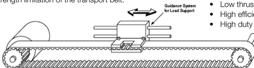
A toothed belt passes around a pulley in each end of the actuator and is attached to the carriage to pull it back and forth along the length of travel. The carriage is supported by a linear bearing system to provide load carrying capacity. The belt is reinforced with steel tensile elements to provide strength and minimize belt stretch. Timing belt systems are a good solution for applications requiring:
