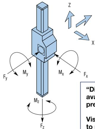
**“DimAxes” software is available for determination of precise carriage loading.**
