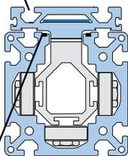
Magnetic strips recessed in the profile ensure that the strip seal is fully sealed with the profile.
