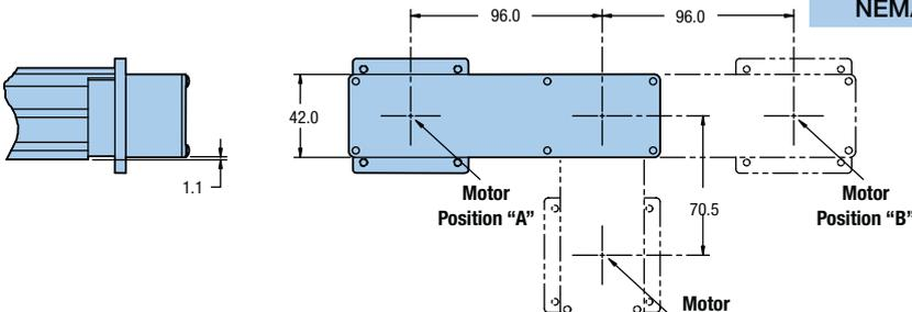
Note: Some sensor pack and encoder restriction apply when mounting motors larger than NEMA 23 in the A or B positions. Please consult factory.
