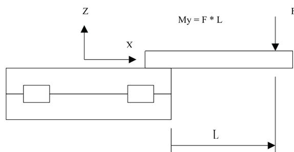
A moment loading defines a twisting load about the bearings. The impact of a moment load is that it is not distributed about all of the bearings uniformly. A moment load can be created in a variety of orientations:
