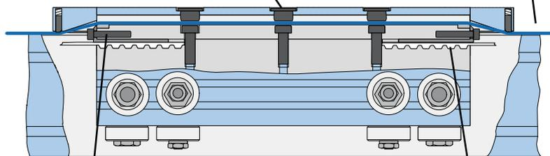
Polymer inlays serve as a bearing surface for the strip seal.
