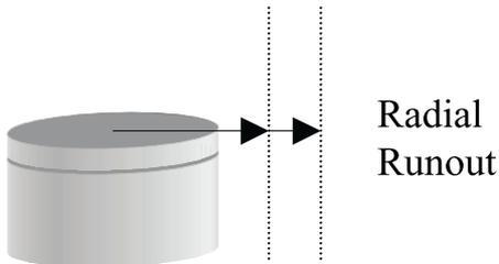
The total indicated reading of the horizontal movement of the rotary table.
