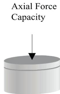
The maximum allowable force acting along the axis of rotation of the rotary stage.
