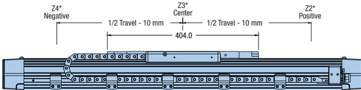
\*Z2, Z3, Z4 shows Carriage Center-line Location for Selected Z-Channel Position
