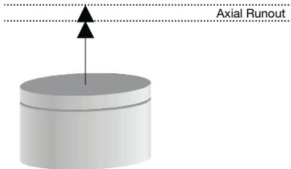
The total indicated reading (TIR) of axis movement along the axis of rotation
