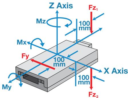
**Fz<sub>1</sub>** is the load applied in the Z Axis direction, 100 mm off end, causing Mx rotation around the X Axis.
