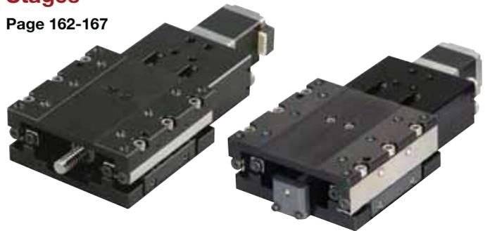
MX80S ballscrew driven motorized stages (left) offer high performance 100% duty operation with higher thrust (128 N) and velocities up to 100 mm/second. Featuring a PTFE coated leadscrew drive assembly (right), the MX80S provides cost-effective linear translation at velocities to 200 mm/second.
