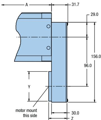
Parallel motor mounting is employed whenever a shorter overall unit length is needed. The motor is positioned along the sides or bottom of the table as designated by position A, B, or C. (No coupling required)
