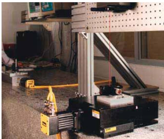
*ZP200 utilized in a laser test set-up*
