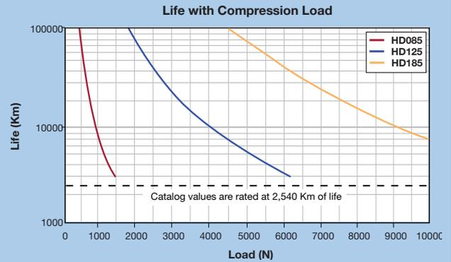
This graph provides evaluation of the support bearing life/load characteristics. The curves show the life/load relationship when the applied load is centered on the carriage, normal (perpendicular) to the carriage mounting surface.
