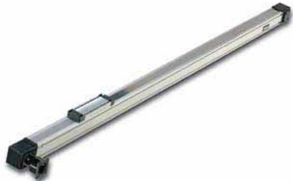
The "SR" series, having a square rail ball bearing system, complement the RB series by providing increased moment load capacities without an increase in profile size. The SR utilizes the same reliable timing belt and pulley drive system found in the RB.
