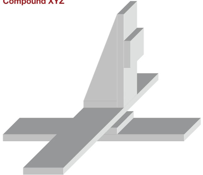
This configuration provides the simplest form of 3 linear degrees of freedom of a positioning system with the smallest footprint. In using this configuration care must be given to calculate the three dimensional accuracy. In particular the Abbe error. (Due to large offset between the bearing of the lowest stage and the point of interest at the top of the vertical stage.)
