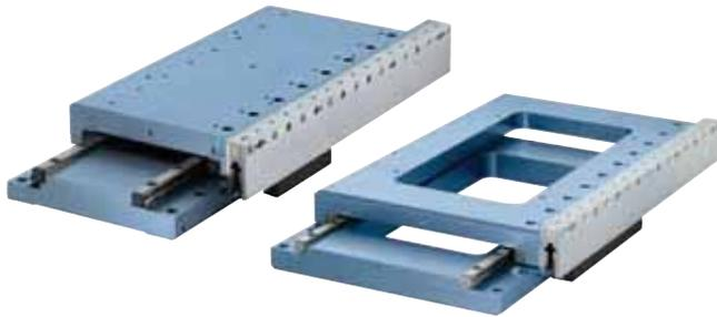
Linear Motor Ultra Stages utilize a non-contact optical linear encoder, integrated directly into the stage footprint. The encoder tape scale is mounted upside-down and referenced directly off the bearing surface, eliminating any Abbe error and protecting it from any debris. The encoder read head is mounted inside the stationary base, eliminating moving wires.
