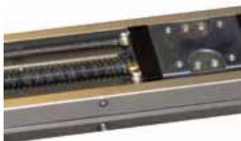
With the steel U channel body and integrated bearing design, the structural rigidity of the 402/403XE is significantly stiffer than most aluminum body positioners. The increased stiffness results in reduced overall cost due to the elimination of support structures.
