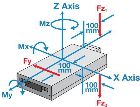
$F_{z1}$  is the load applied in the Z Axis direction, 100 mm off end, causing  $M_x$  rotation around the X Axis.
