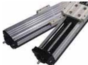
For added protection to the bearing system and drive train, an optional hardcover is available. This will bring the positioner to an IP20 rating and prevent large particles from entering and damaging the screw or bearings.
