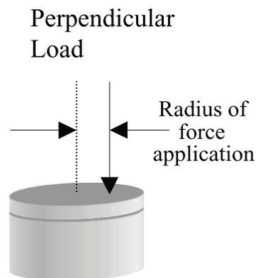
The maximum load perpendicular to the positioning stage top surface, applied at a specified radius from the axis of rotation of the table.
