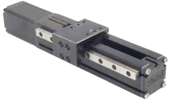
Designed for OEMs needing simple positioning solutions for instrument and light industrial applications, the PROmech family of positioners offers a complete positioning solution at a price OEMs can afford to design into their equipment. The LP 28 provides travels from 5 mm to 500 mm; the LD28 provides travels from 5 mm to 300 mm. Both products feature an anti-backlash nut for excellent positioning.
