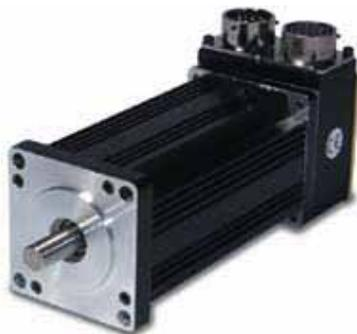
The SM Series brushless servo motors feature a slotless stator design that eliminates all detent torque in the motor, allowing the motors to provide extremely smooth motion, especially at low speeds. This design is also ideal for applications involving high-inertia loads (such as lead screws and belt drives).
