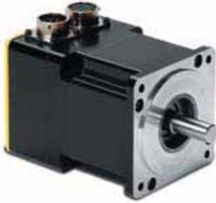
The BE Series brushless servo motors produce high continuous stall torque in a cost-reduced package. The increased torque is the result of eight magnetic poles on the rotor instead of the four poles traditionally found on motors in these frame sizes.
