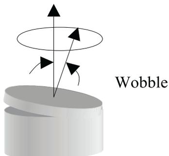
The angular error between the actual axis of rotation and the theoretical axis of rotation.
