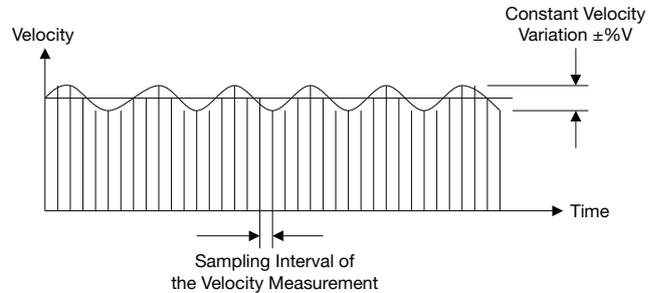
Typically measured in percent variation from a nominal value at a given sampling interval. High smoothness of motion can be achieved by using crossed roller or air bearing stages with ironless linear motors.
