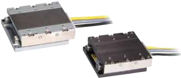
MX80L stages provide high-precision positioning and linear motor dynamics for positioning light loads within a small workspace. They offer exceptional straightness and flatness of travel, and can position repeatedly within  $\pm 0.4$  microns with encoder resolutions down to 10 nanometers.
