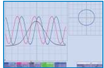
Sine-wave output signals from transducer.
