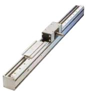
The "endless" linear unit is designed for positioning payloads over long travel distances with high rigidity and repeatability. This is accomplished by incorporating Parker's uniquely designed rack-and-pinion based drive system with the RB series roller wheel bearing system.
