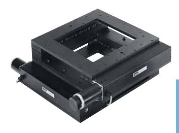
Table elements are constructed of high quality aluminum alloy and are protected with black anodized surface finish. The top and bottom mounting surfaces are precision machined to assure flatness, and fixturing holes are fitted with locking steel threaded inserts. These units are offered in English or metric versions, and in two grades: precision grade and standard grade which permit cost savings to be realized in less demanding applications.
