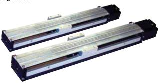
The steel base constructed 402/403XE series offers rigid compact positioning for the cost conscious motion applications. A highly integrated ballscrew, bearing retainer system results in a very low overall height and high payload capacities.
