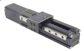
Designed for OEMs needing simple positioning solutions for instrument and light industrial applications, the PROmech family of positioners offers a complete positioning solution at a price OEMs can afford to design into their equipment. The LP 28 provides travels from 5 mm to 500 mm; the LD28 provides travels from 5 mm to 300 mm. Both products feature an anti-backlash nut for excellent positioning.
