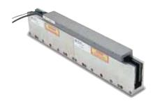
Parker Trilogy's I-Force ironless motors offer high force and rapid accelerations in a compact package. Parker Trilogy's patented I-beam shape, with its overlapping windings, allows for a higher power density in a smaller motor, improved heat removal, and added structural stiffness. A forgiving air gap and no attractive forces allow for easy installation and zero cogging during motion.
