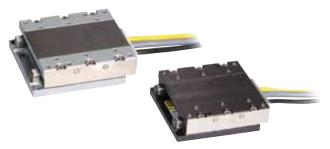
MX80L stages provide high-precision positioning and linear motor dynamics for positioning light loads within a small workspace. They offer exceptional straightness and flatness of travel, and can position repeatedly within  $\pm 0.4$  microns with encoder resolutions down to 10 nanometers.
