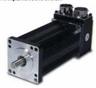
The SM Series brushless servo motors feature a slotless stator design that eliminates all detent torque in the motor, allowing the motors to provide extremely smooth motion, especially at low speeds. This design is also ideal for applications involving high-inertia loads (such as lead screws and belt drives).
