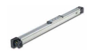
These are the most popular electromechanical modules in the Parker line. They utilize a unique composite roller wheel bearing design coupled with a timing belt and pulley drive mechanism to provide long travel with high speed and high acceleration.
