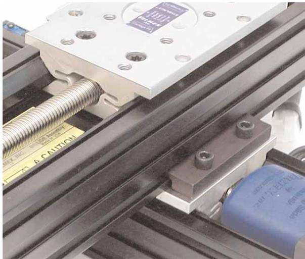
**Left: Rigid XY attachment using BiSlide cleat.** The Y axis can be positioned anywhere on X axis without an adapter plate or special holes. *Items needed:* Two MC-2 cleats and four MB-1 bolts.
