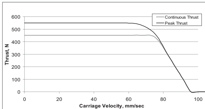
HLD60 Twin Rails - SM23165DT @ 24V, 2.5mm/rev
